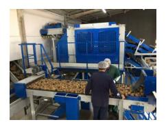
process, ensures that the fall-through dimension remains the same at all times. The dimensional accuracy has a maximum deviation of plus or minus 0.2 mm (uncovered screen) and 0.5 mm (rubber-covered screen). For extra-sensitive varieties and optimum product-friendliness, DT Dijkstra offer rubber-covered or full rubber screens. The screens are produced in-house according to the highest quality standards.
