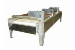
Various techniques are available for dry cleaning tuberous and bulbous products (potatoes, beetroot, etc.). The choice of system is determined by the customer's desired result. In each case, minimising damage to the product during cleaning has priority.
